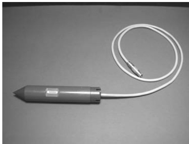
FIGURE 4 – AC corrosivity probe based on modified high-resolution ER principles.
