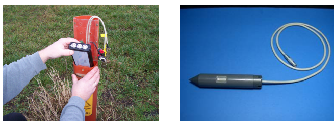
FIGURE 4 – Devices for AC corrosion detection and mitigation installed in standard measuring posts (left), and the probe used for AC corrosion detection (right).
