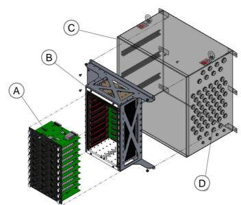
The MCCM is designed for offshore installation inside the transition piece or similar confined space. The system is configurable, depending on requirements to the specific measurement campaign.
