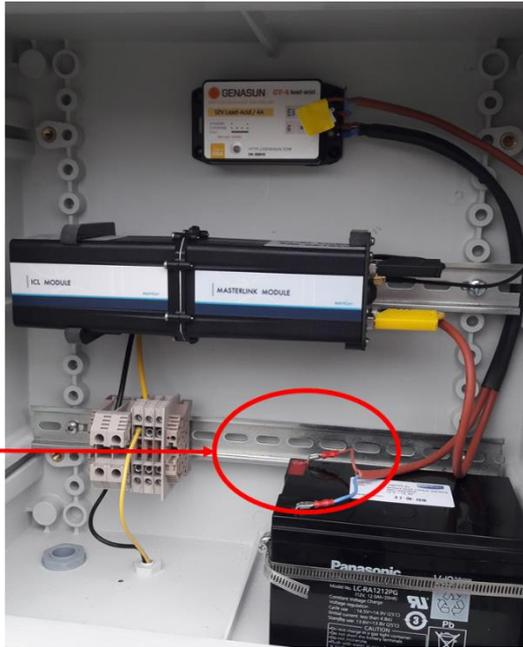
Step 2: Connect the Solar Charger to the solar panel
