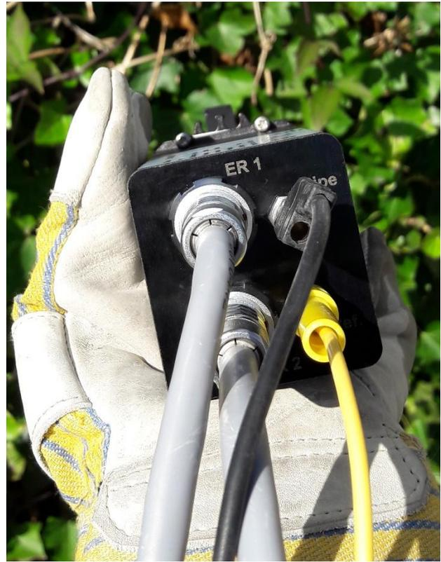
Figure 10C: ER, Pipe and Reference Cables after connection
