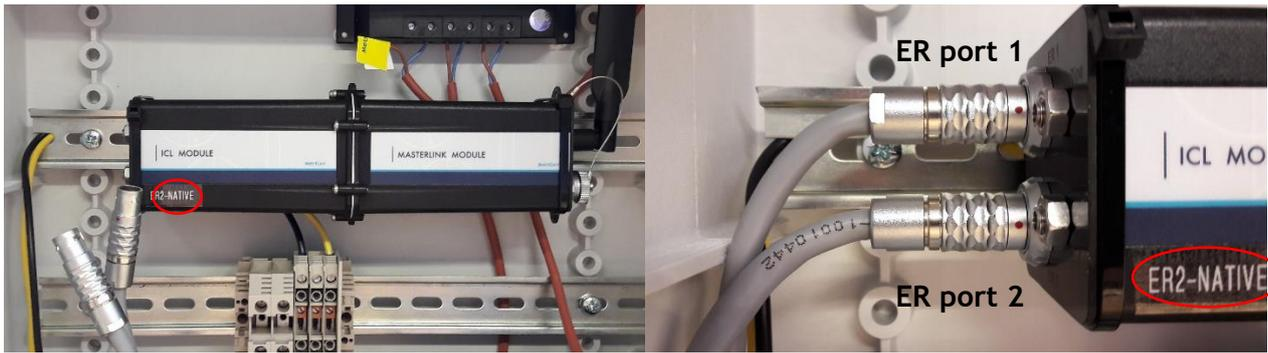
2. Connect the probes to the desired ports. The connector will only engage when the red dots are facing forward (as pictured Figure 8c, above).
