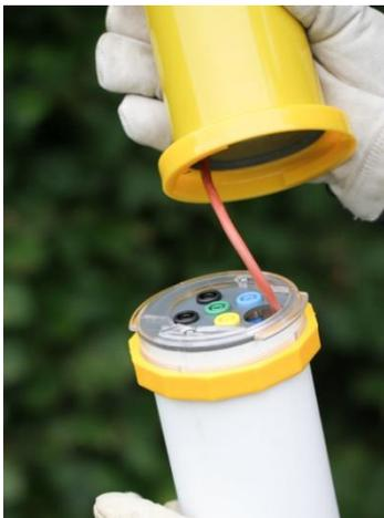
The MetriCorr Big Fink Battery requires only that the power cord is connected to connector H (Figure 3), as per **step 4**, above. Once power is connected ensure that the logger is ON and set up correctly (see **Section 3**).
