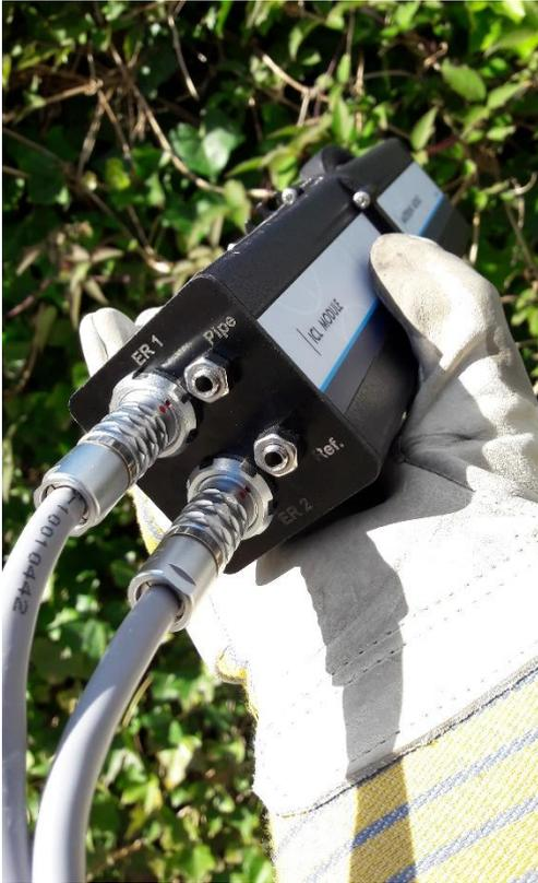
Figure 10b: ER Probe Cables after connection (note red dots line up)
