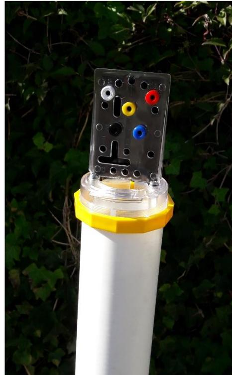
6. All additional cables should be correctly terminated on either the standard Big Fink terminal board (in the case of the Solar Hat Solution), or on the supplied modified (flat) terminal board in the case of the hat battery solution (see Section 4.2.2).
