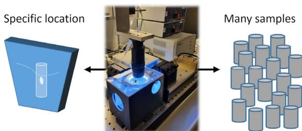
Figure 1. A custom built  $\mu$ -lathe is incorporated in two separate workflows to prepare cylindrical bone samples from specific locations within the whole-bone context (left) and for consistent high-throughput sampling of many specimens for comparative studies (right).
