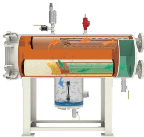
Typical Horizontal End Opening Coalescer Separator Flow Diagram for Fixed Installation (including optional accessories)
