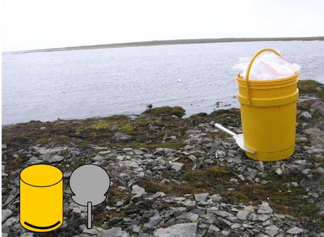
Figure 4. Peltipelle-sampler on the shore of Kapp Linné pond. The sampler is composed of a bottomless bucket and a metal paddle. Photo taken by Anni Pulkkinen.
