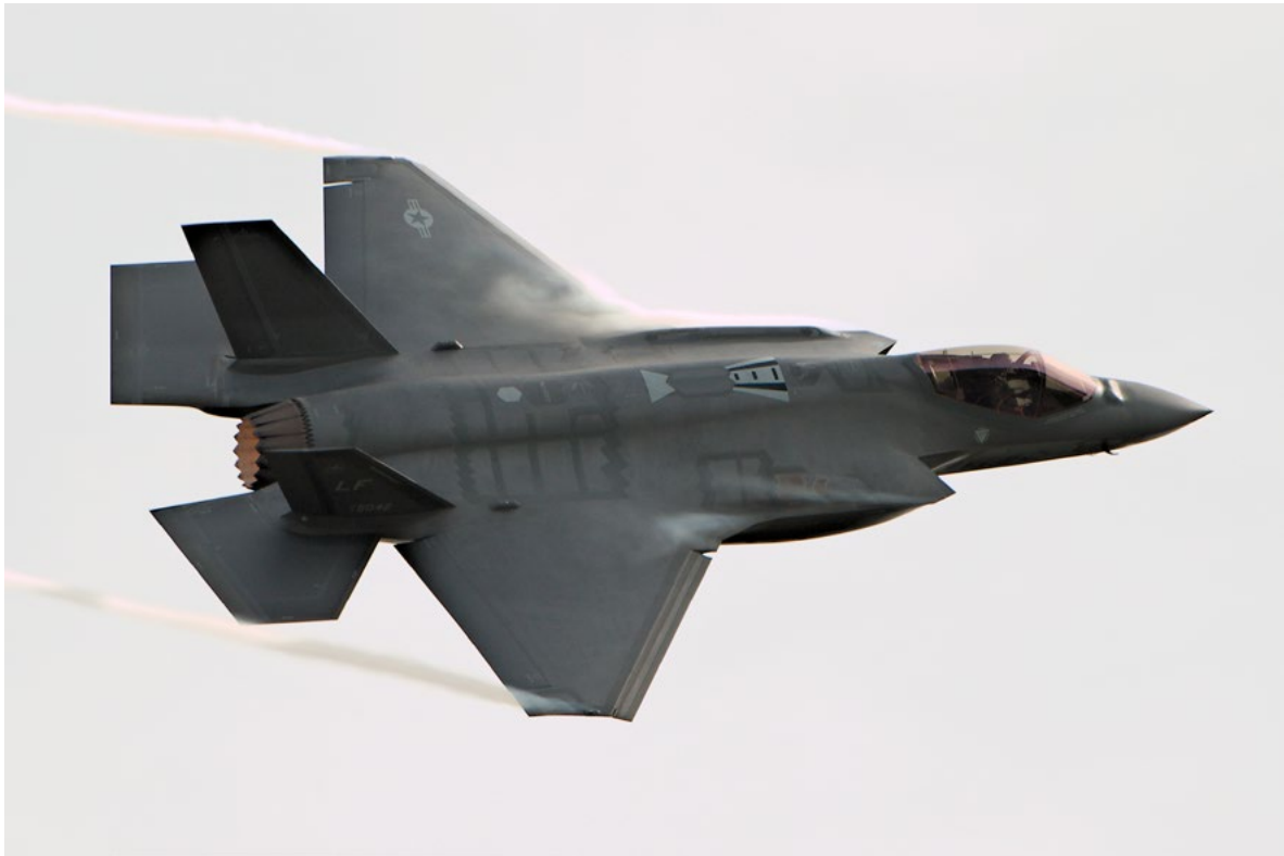
F35-A fighter jet consumes about 5,600 litres of oil per hour of flight. Credit: Airwolfhound/Flickr (CC BY-SA 2.0)
