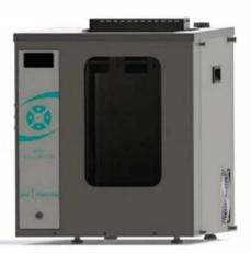
The EVS Viscometer bath comprises of a stainless-steel inner tank with double glazed front window. The window is illuminated from the front with LED lighting.
