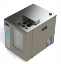
A five-button control pad on the EVS provides single step access to menus. The user interface includes selection of set-point, reference temperature (offset), units (°C, °F) and the chiller set-point.
