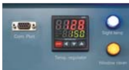
Electronic over temperature shutdown system.
