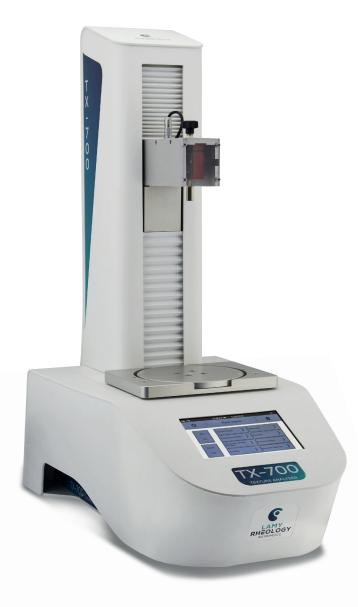
With its wide range of probes and fixtures, the TX 700 is the ideal tool for your texture analysis. Thanks to its touch screen directly displaying the curves, its method programming capability, storage and analysis of measurements, the TX 700 will fit in laboratory and production area.
