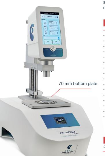
The motorized lift of the RM200 CP4000 PLUS allows a fast and repeatable installation of cone and plate measuring systems guaranteeing reliable rheological measurements whatever your application.
