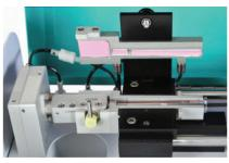
Thread the syringe into the measuring cell and close the thermal jacket
