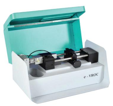
*e*-VROC<sup>™</sup> provides extensional viscosity data by monitoring the sample flow through a microfluidic contraction within the measuring cell. The system measures the pressure upstream and downstream of a contraction using the MEMS pressure sensors, and it registers changes in the flow. The fluid undergoes an almost constant extension through the contraction/expansion, enabling the calculation of the extensional viscosity.
