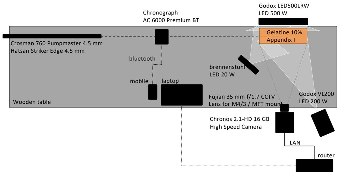
Figure 1: Principal sketch of test arrangement for 4.5 mm calibre gelatine 10% experiments.
