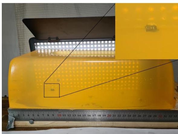
Figure 3: Terminal ballistic photo of GB210828nr3 after shot 1 and shot 2 at time 14:59 for Sphere and Dome mm with shot 1 and shot 2 having 182.0 and 132.7 m/s in impact velocity resulting in DOP 9.0 and 7.8 cm, respectively. Zoomed in area in figure shows shot 2.
