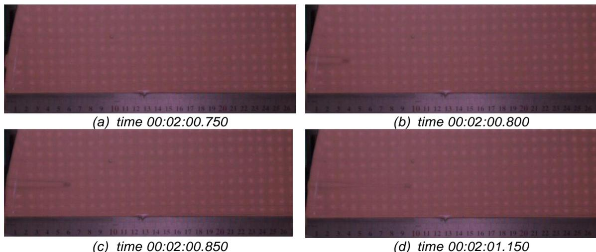
Figure 5: Chronos 2.1 camera capturing 10 000 FPS of dynamic cavity and penetration at different times (a) to (d) for Dome 4.5 mm with 132.7 m/s impact velocity into gelatine 10%. Test series GB210828nr3 shot 2. The unit of the metallic ruler below gelatine is in [cm].
