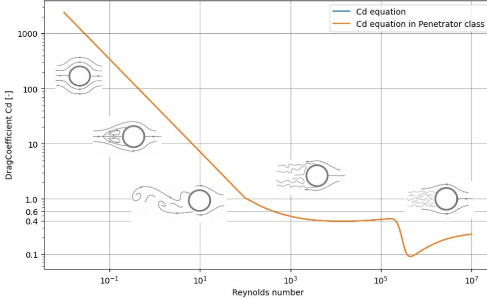
Figure 6: Drag Coefficient as a function of Reynolds number, equation (4), including illustration of different flow regimes, illustrations from [8].
