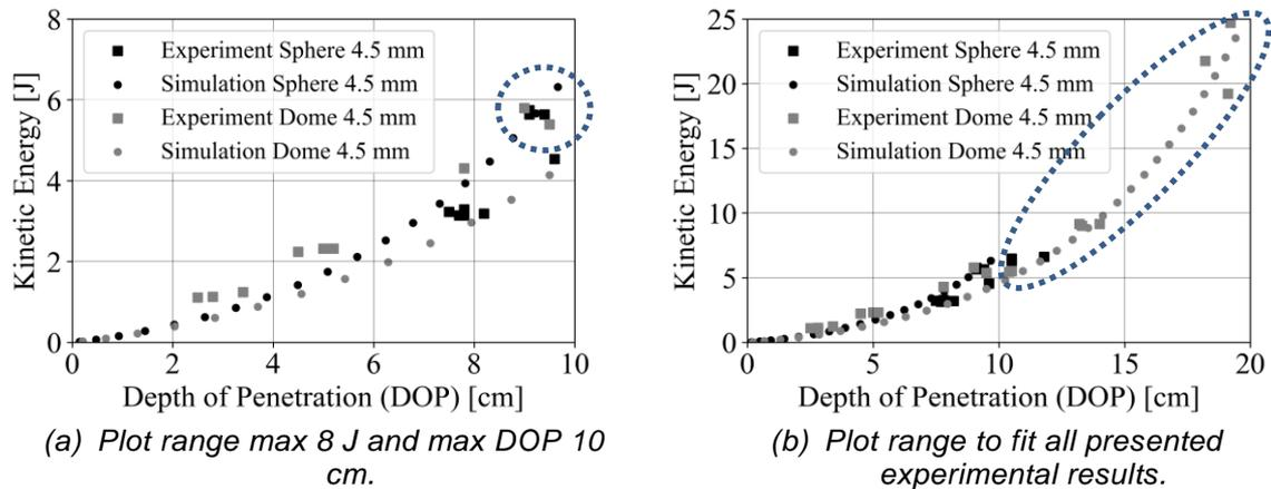
Figure 8: Maximum Kinetic Energy as a function of DOP for Experimental data of Sphere and Dome compared with simulations.
