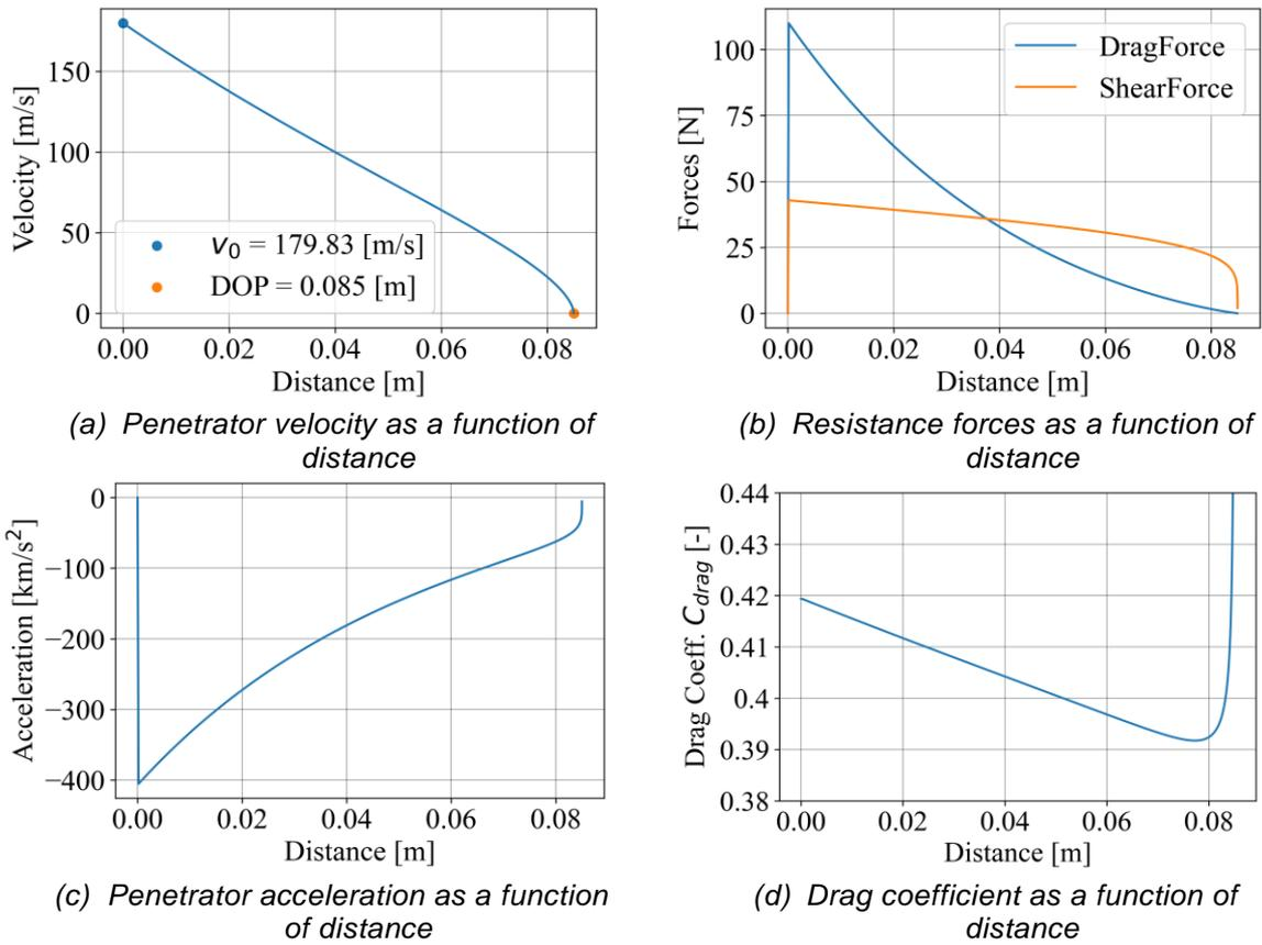
Figure 7: Simulation of FBI protocol requirement in gelatine block 10% with  $v_0 = 179.83$  m/s resulting in DOP 8.5 cm.
