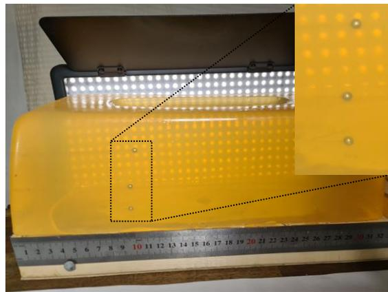
Figure 2: Terminal ballistic photo of GB210827nr2 after shot 3 at time 16:06 for Sphere 4.5 mm with 181.3 m/s impact velocity into gelatine 10%. DOP 9.1 cm, top, middle, and bottom sphere in the picture corresponds to shot 3, shot 2, and shot 1, respectively. All three shots fulfil the FBI protocol requirements of DOP range. Zoomed in area in figure shows all three shots.
