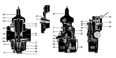
until the float just contacts the float needle. In this position the tongue on the float hinge is set in such a way that the flat surfaces at the bottom of the floats are parallel to the washer surface of the float chamber.
