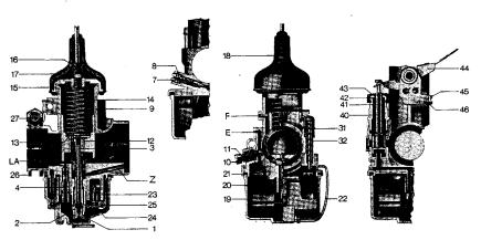
This initial mixture then flows through the idling outlet bore into the bore where it is mixed further by the main airstream.
