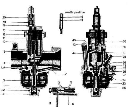
space in the float chamber (26) through which the fuel flows from the float chamber to the main jet. This ensures that fuel is not spun away from the main jet under particularly severe operating conditions.
