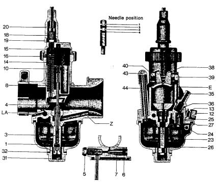
When fitting a new float, the fuel level has to be adjusted. When doing this, the spring-loading of the float needle should be taken into account which must not be compressed by the float weight when making the adjustment. It is therefore advisable to hold the carburettor in a horizontal position until the float just contacts the float needle. In this position the float hinge is bent in such a way that the top edge of the float is parallel with the top edge of the float chamber.
