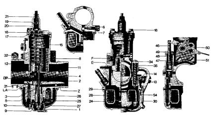
supply any fuel. This is then supplied via an auxiliary system, the idling system, which consists of the idling jet (5) and the mixture control screw (6) with sealing ring (7) which acts as a seal for the screw and also stops it from working loose.
