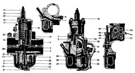
It is therefore advisable to put the carburettor in a horizontal position until the float just contacts the float needle. In this position the pointer on the float hinge is set in such a way that the float top edges are parallel to the top edge of the float chamber.
