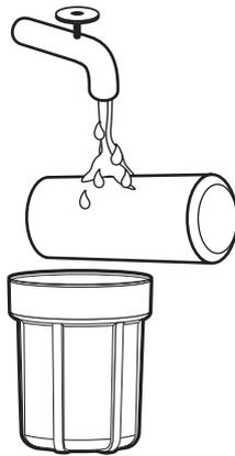
Rinse the filters in water to remove particles or discard and replace them when they are worn out.
