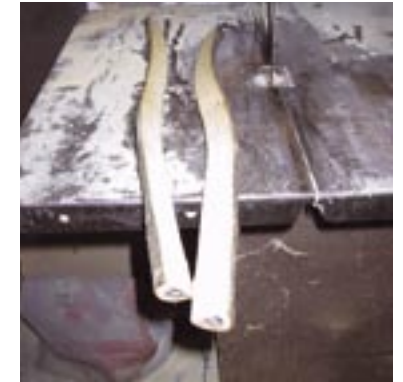
The whole tree is cut up in manageable pieces, and brought to the carpenter's workshop, to be cleaved on the band saw
