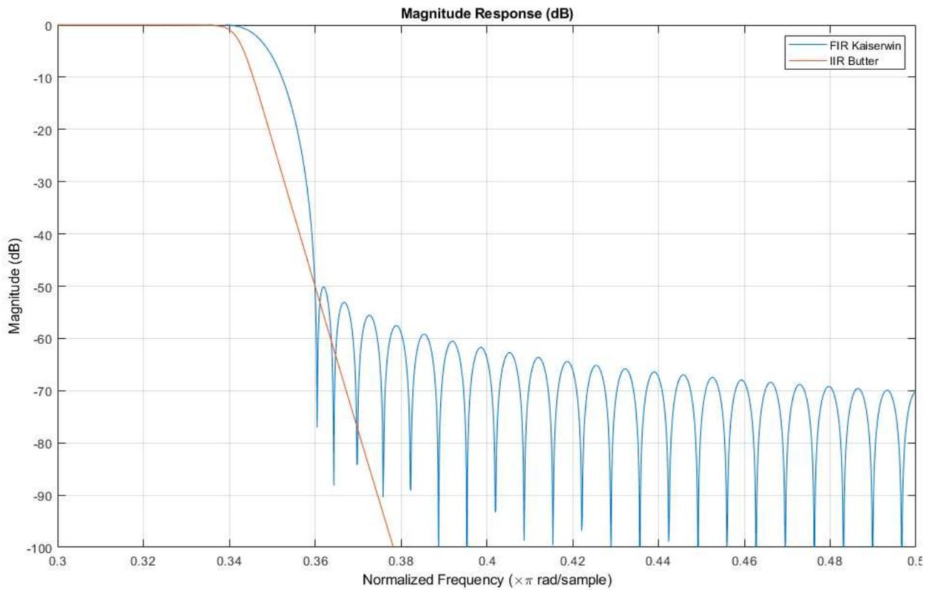
**Take the filter object and integrate it into SIMULINK by the System Design environment (optional)**
