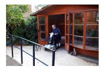
The floor of the summerhouse was strengthened to support the weight of scooters and a shelf with seven charging points was installed. Automatic PIR lighting ensured that users did not have to reach for light switches when entering and leaving the facility. Outside the summerhouse a new concrete apron was laid to help with access and to make manoeuvring easier for scooter users. And finally, the garden
