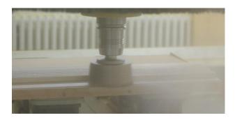
Tool prisms rebate cutter Leuco P-System D = Ø86 mm, Z = 3
