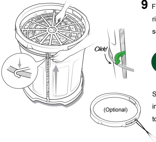
Secure the unit to the wall – (optional) Secure in the corner of the stable with enough room to get your hand around to unclip regulator.
