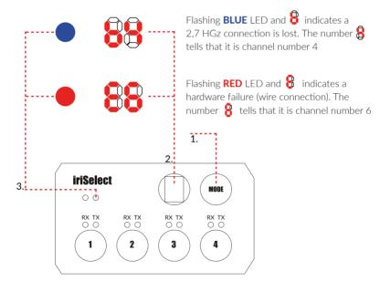
By pressing the MODE button (1) error messages can be reset, and MODE selection will reappear. Loss of wireless connectivity is described under TROUBLESHOOT 4.1
