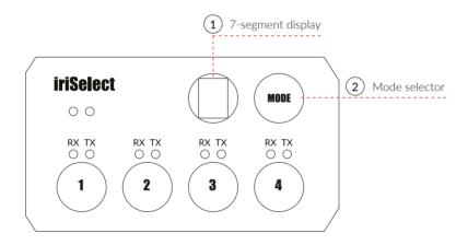
When toggling through MODEs (1) the selected MODE (2) will be uploaded 1 second after the button is released. When the selected grid is uploaded to iriSound, a dot will appear in the lower right corner of the Display
