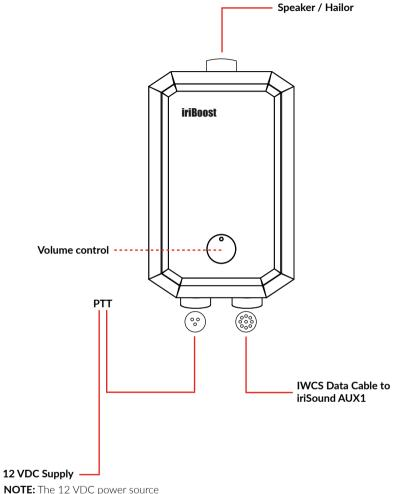
**NOTE:** The 12 VDC power source and the iriSound MUST have common ground.
