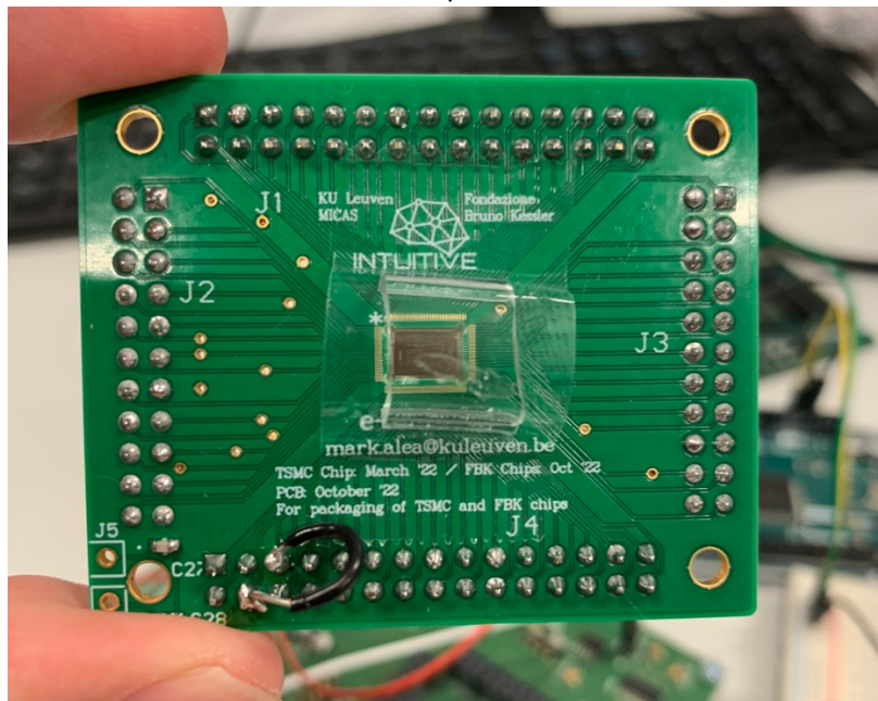
Figure 11. a) To reduce the chip bondwires for increased robustness during mechanical contact, the area where the chip is to be bonded to the package PCB is milled by 0.8 mm (same chip thickness). b) Image showing the actual readout chip bonded on the package PCB. The chip contains 100 pads in total: 52 (optional external AER interface), VDDPST-5V (2), VDD-1.8V (2), AVDD-1V (2), LCVDD-1V (1), DVDD-1V (2), GND (5), AER interface (12), serial interface (4), current biasing (1), voltage biasing (2), spike generation parameters (8), analog output for debug (2), calibration (2), digital configuration bits (2), and poling mode enable (1).
