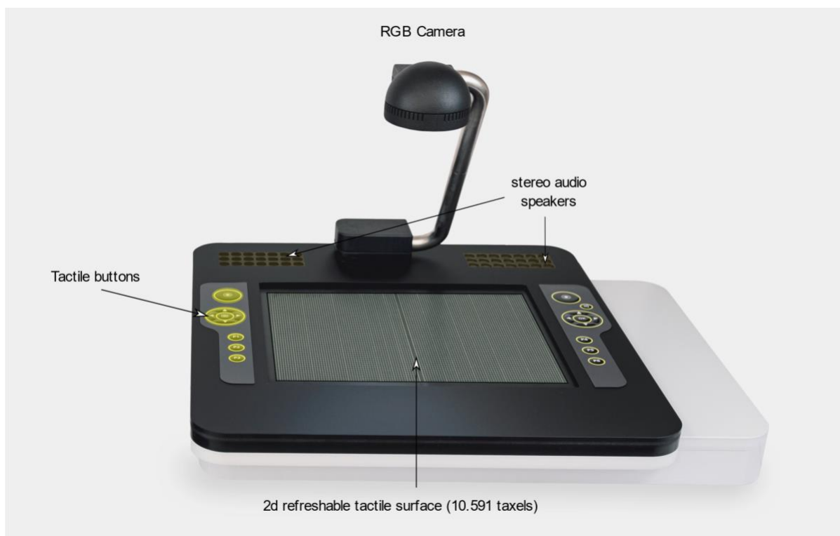
Figure 5- Tactonom device input/output characteristics overview.
