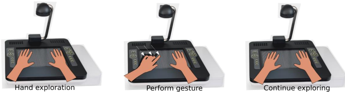
Figure 7 - Execution operation UI alternatives in 2DRT devices, (Tactonom process).
