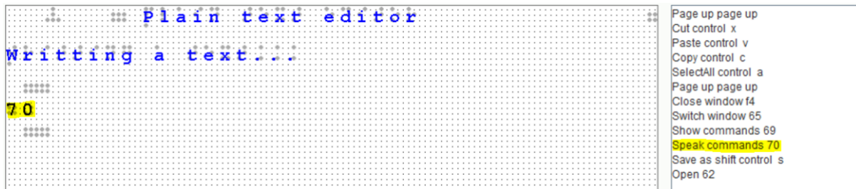
Figure 9 - Tactonom Text editor - commands presented on the right side of the image. The user fails to execute the command: "Speak commands" since the current focus is on a text box, which receives all text information from input keyboard.
