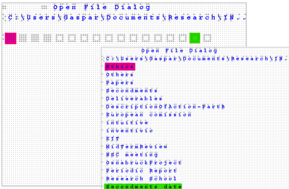
Figure 12 - Tactonom File Explorer - Representation of files with textures (left) and with braille lines (right)
