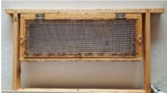
Figure 4. Impression of the APITrap, note the hinge and swivels to close the trap when in use.
