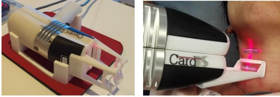
Figure 1. (a) The CARDIS handheld LDV sensor with 2 x 6 beams at 1550 nm. The LDV sensor is developed in CARDIS project. (b) The measurement position of the LDV sensor for local-carotid PWV measurement. Reproduced from [3]
