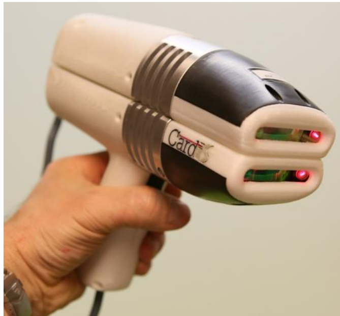
CARDIS prototype medical device that can perform Laser Doppler Vibrometry on a patient's skin to deduce metrics for arterial stiffness and to diagnose cardiovascular diseases
