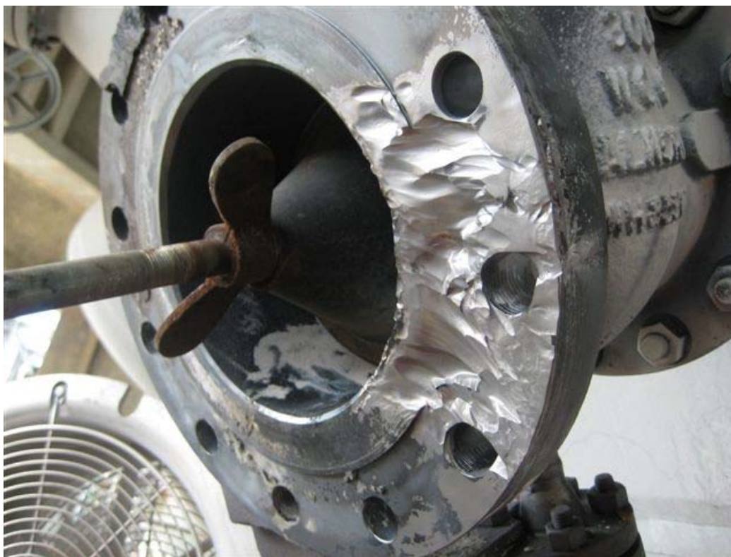
Figure 4-43 – Erosion Corrosion of a 1.25Cr 300 # valve flange on an FCC Catalyst withdrawal line.
