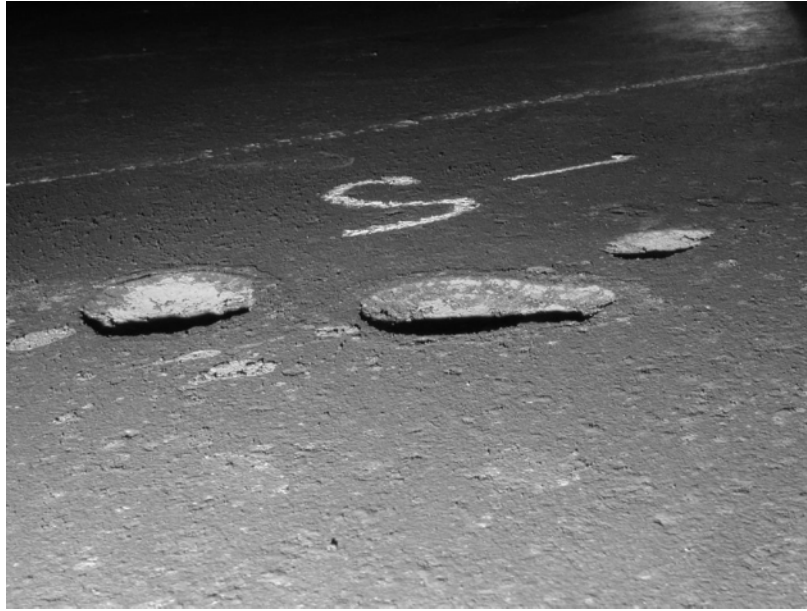
Figure 4-89 – MIC of diesel tank bottom.
