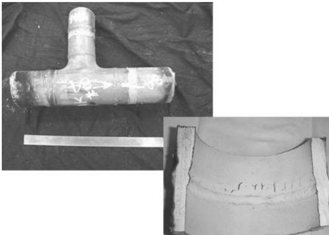
Figure 5-55 – A 3 in x 4 in (76 mm x 100 mm) diameter tee in a hydrocarbon line off a water knockout pot in the FCC light ends recovery section. Cracking developed after 6 months service.
