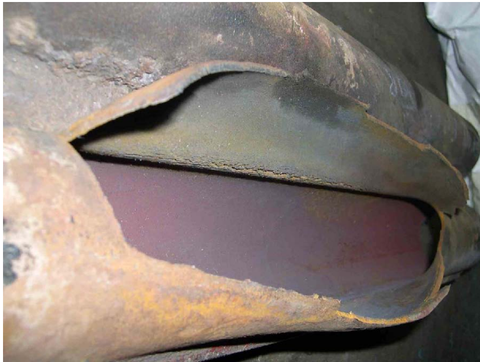
Figure 4-141 – Corrosion fatigue failure of a boiler tube.
