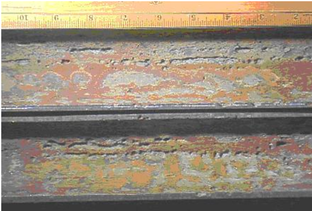
Figure 4-85 – CO 2 corrosion of a carbon steel oil and gas production flow line.
