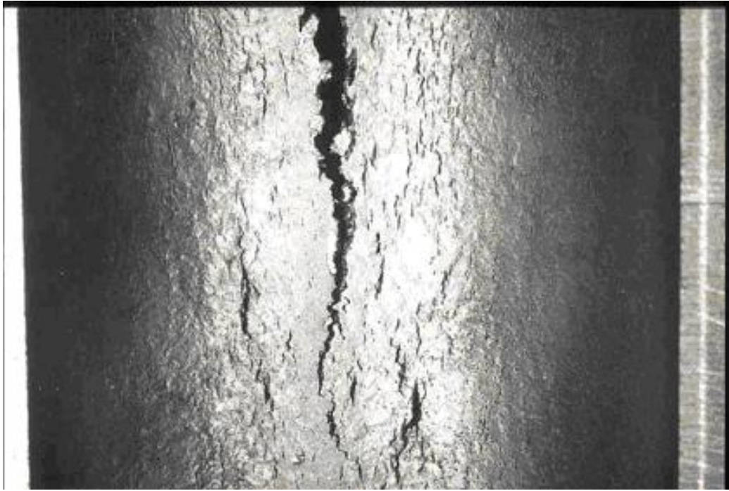
Figure 4-18 – Creep rupture of an HK40 heater tube.
