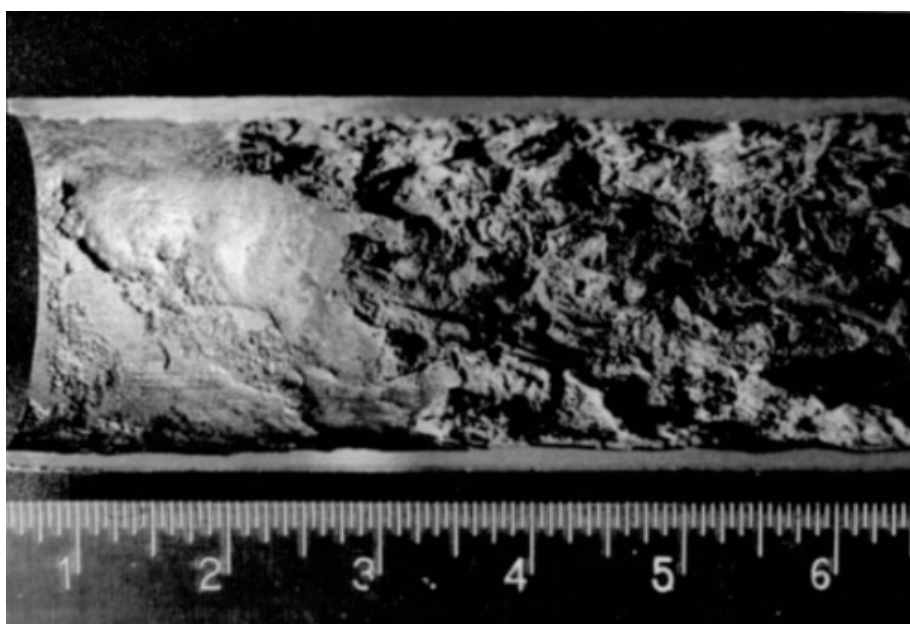
Figure 4-83 – General metal loss (left end of tube) on steel resulting from oxygen corrosion. The color of hydrous ferric oxide is orange to red brown.
