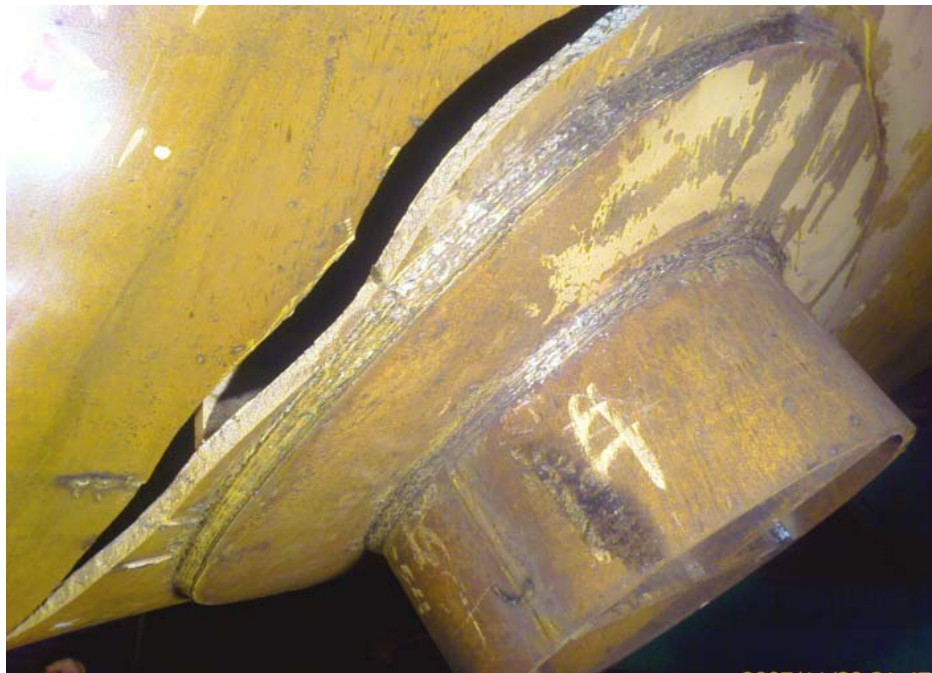
Figure 4-15 – Brittle Fracture of vessel shell during hydrotest.
