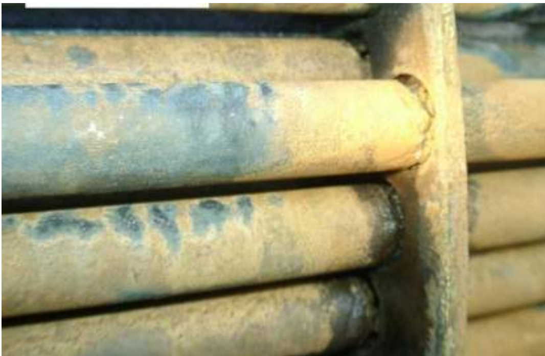
Figure 5-22 – Accelerated corrosion under a baffle.
