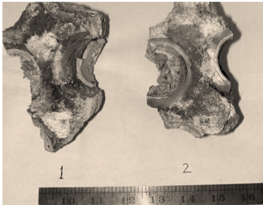
Figure 4-59 – Damaged refractory and ferrules.
