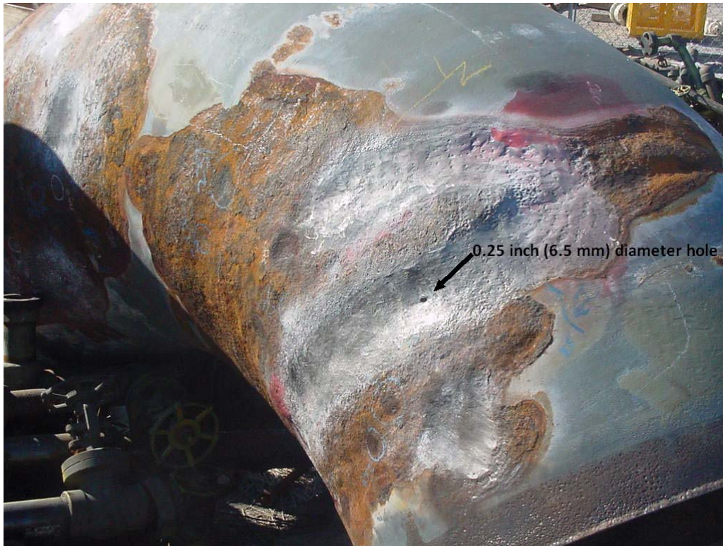
Figure 4-75 – CUI of a 30 inch CS Butadiene line showing highly localized corrosion which could only be found by stripping the entire line. Note the 0.25 in (6.5 mm) diameter hole at arrow.
