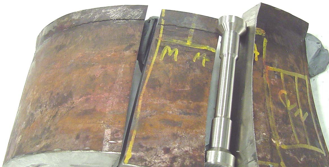
Figure 4-60 – Samples removed from a cracked 12-inch NPS 321SS elbow in hot recycle H 2 line that operated at 985°F in hydrocracker.
