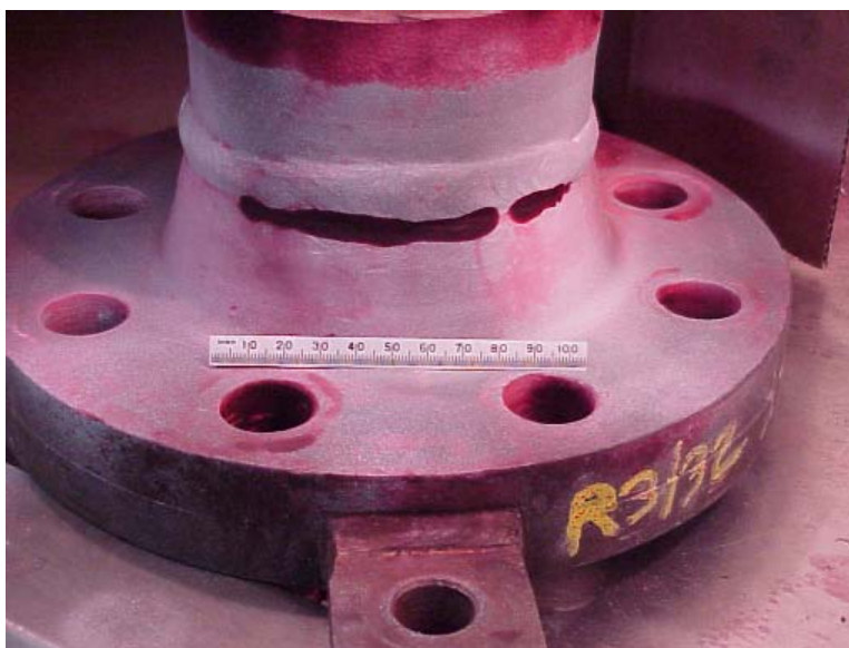
Figure 4-41 – Failure of nickel alloy DMW joining HP40 (Nb modified) tube to 1.25Cr-0.5Mo flange in a Steam Methane Reformer due to cold hydrogen disbonding of the buttering layer. Process temperature 914°-941°F (490° to 505°C), Pressure (2.14 Mpa), H 2 content 10-20% (off-gas).
