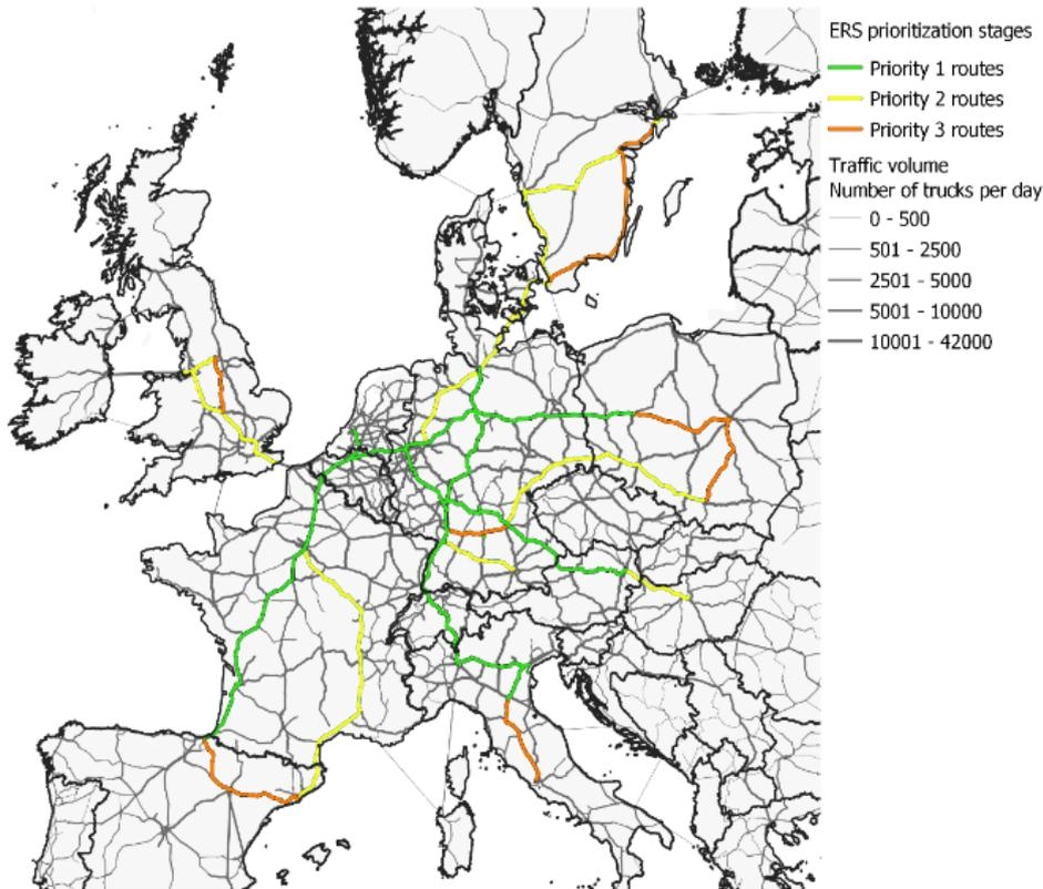
Figure II. Potential EU-wide extension stages of ERS in Europe. Own illustration based on (Speth et al. 2022b)
