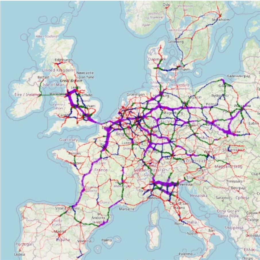
Figure 12. HDV traffic intensity on the main European roads. Own illustration based on (Speth et al. 2022b). violet: top 10 % of mostly used roads, i.e., top 10 % of number of HDV per day per road segment) in dark blue: top 10 – 20 %; dark green: top 20 – 30 %; red: remaining roads in red; width of the lines: number of trucks per day per road segments.
