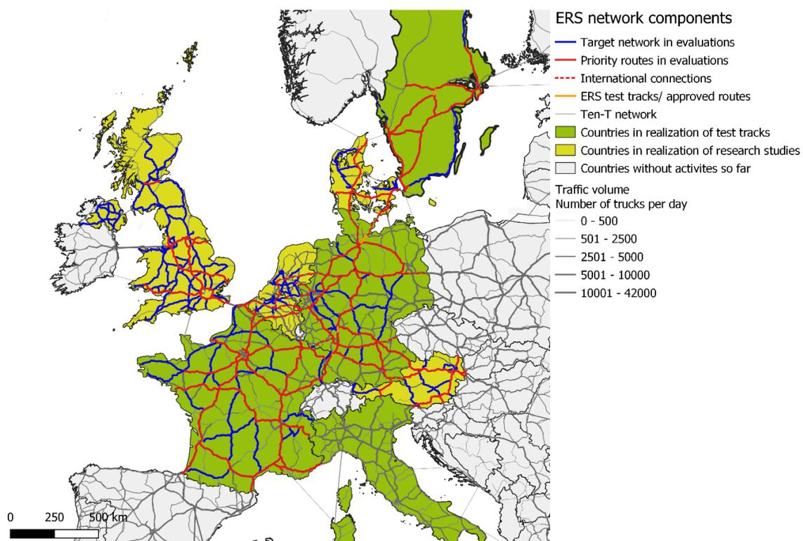
Figure I. ERS on European route network based on national ERS studies. Source: Own Illustration based on: Speth et al. (2022). Traffic volume database by Fraunhofer ISI. TEN-T network database source European Commission - DG Move - TENtec Information System (2022)
