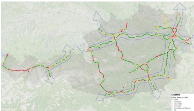
Figure 14. Assessment of the suitability of individual sections of the Austrian highway network for the installation of ERS; green = no limitations, yellow: some limitations, orange: serious limitations, red = almost impossible. Source: Austrian Energy Agency 2022).
