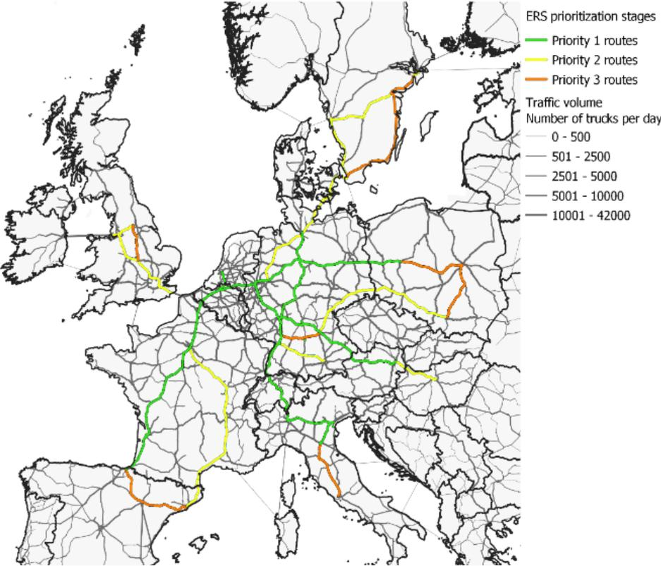
Figure 13. Potential EU-wide extension stages of ERS in Europe. Own illustration based on (Speth et al. 2022b)
