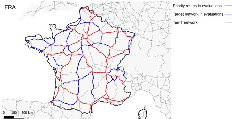
Figure 5. ERS target network and potential priority routes and partial networks in France. Source: Own Illustration based on (RGRA 2022). Ten-T network data by European Commission - DG MOVE -TENtec Information System (2022)
