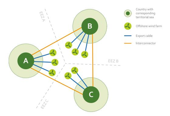
Figure 2. Radial connections.
