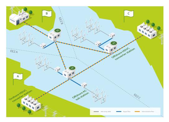
Figure 8. A meshed offshore grid. Source: Baltic InteGrid
