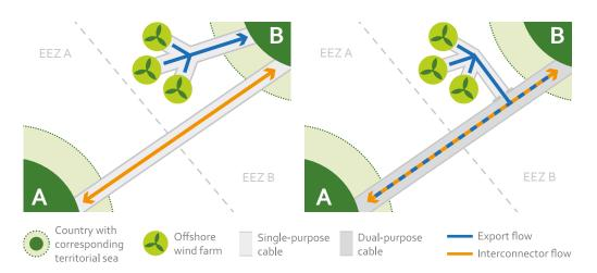
Figure 10. Dual-purpose cable in a meshed grid constellation. Source: IKEM (2018)
