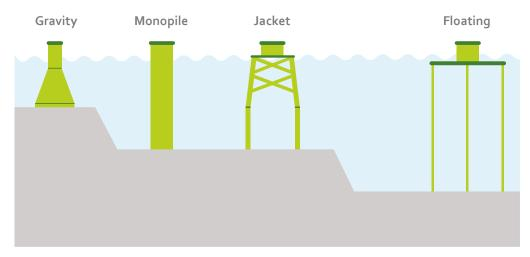
Figure 9. Offshore wind turbine foundations. *Source: Baltic InteGrid*
