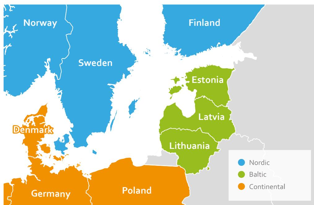
Figure 4. Synchronous grids in Europe.
