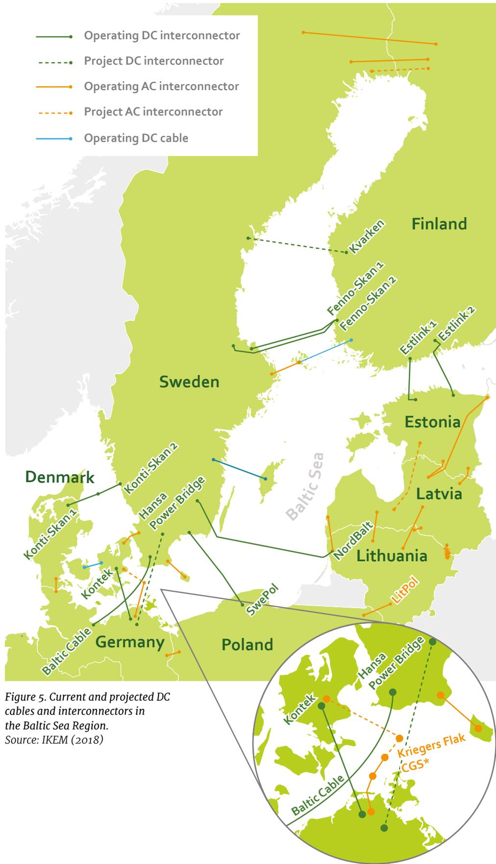
Figure 5. Current and projected DC cables and interconnectors in the Baltic Sea Region.
