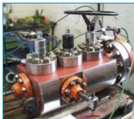
Solid block Xmas tree on test rig
