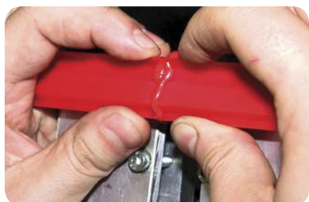
Step 4: Visual inspection of weld
