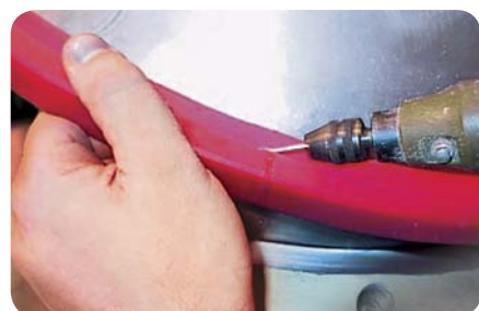
Step 5: Post-processing with special milling tool
