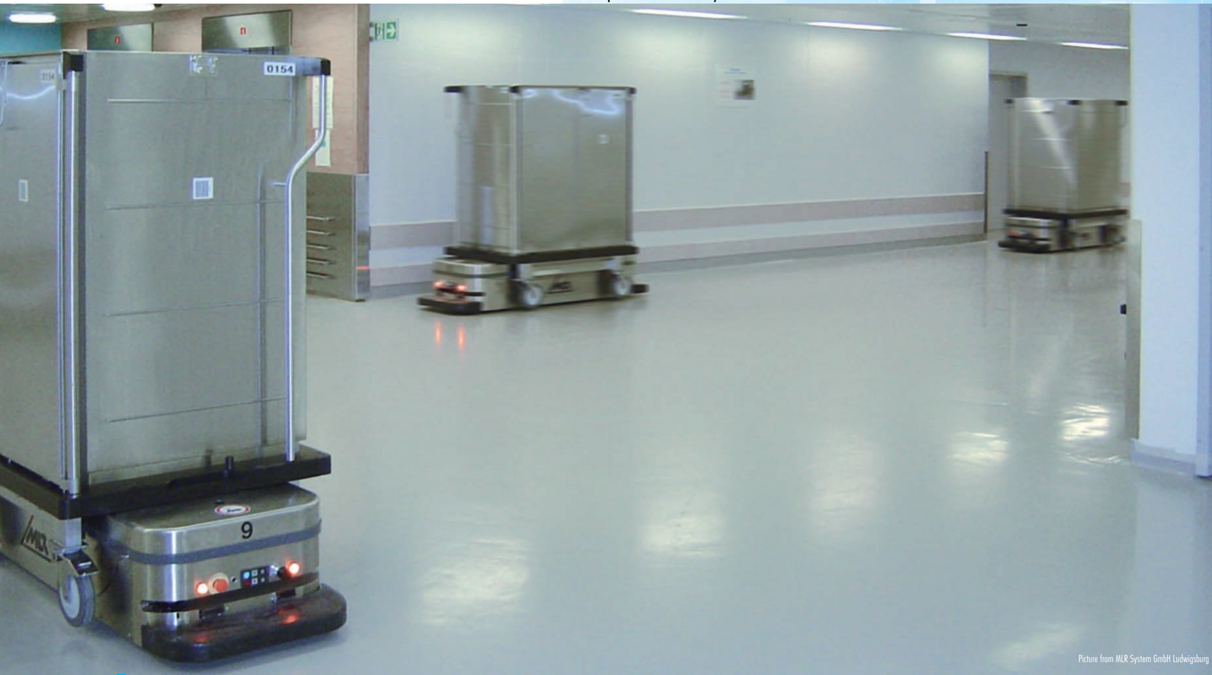
Automated trolley transportation, ground-based with driverless transport system
