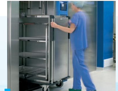
Pushing a transport trolley into a washing system
