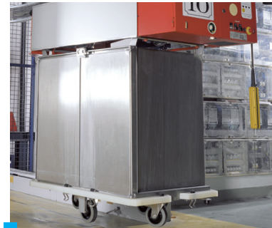
Automated trolley transport, suspended on the top-mounted electric conveyor
