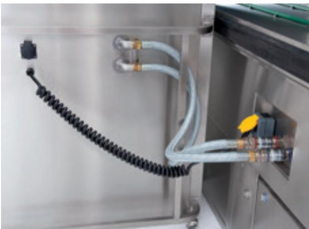
*Flexible hose connections enable variable positioning of the Coolports® along the conveyor belt.*
