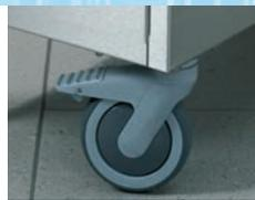
All HUPFER® brand stacking appliances are equipped with corrosion-resistant and maintenance-free plastic castors according to DIN 18867-8 which are mounted in ball bearings. 4 castors per appliance, 2 of which are lockable. Ø 125 mm. The load-bearing capacity of each castor is 100 kg.
