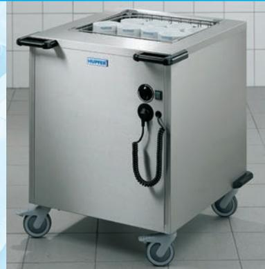
Basket stacker KOUH/50-50 (heated by circulating air). Stacking platform: plastic-coated refined steel basket, 500 x 500 x 150 mm - can be included in the stacking capacity. In addition 7 baskets, 115 mm high or 10 baskets 75 mm high can be inserted. The stacking platform can be removed easily for cleaning.
