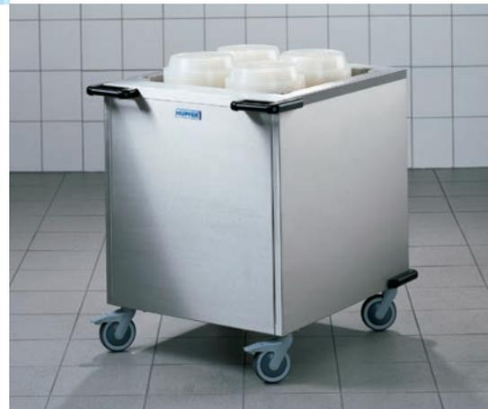
The platform stacker BDUH/60-60/4-S which is heated by circulating air is provided especially for holding portions of hot food on a food distribution belt and subsequently transporting this warm food. It is operated by means of an ergonomic knob, the gradual thermostatic control between 20°C and 110°C can be adjusted in 4 power ranges. A maximum crockery temperature of 80°C is achieved very quickly by the high-powered heating by circulating air.
