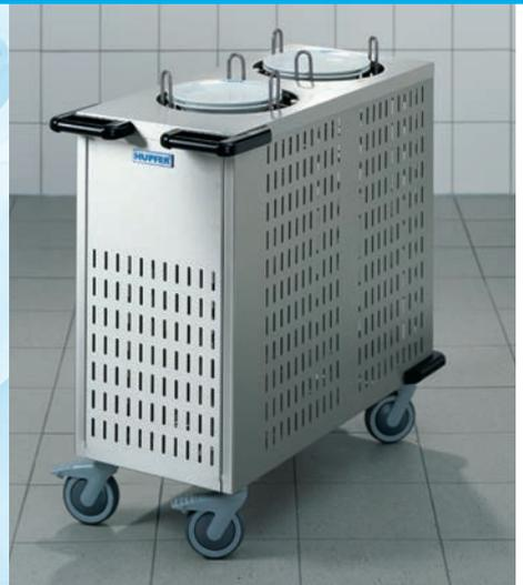
Plate stacker TE-2/VK 19-26 (unheated). Especially suitable for holding portions of cooled food components in Cook & Chill kitchens. The cooling slots ensure rapid exchange of the initially warm stacker atmosphere for the cold air in the cold store and ensure the low temperature is uniformly distributed throughout the crockery. An additional area of use is for the portioning of cold food for distribution in Cook & Serve kitchens.
