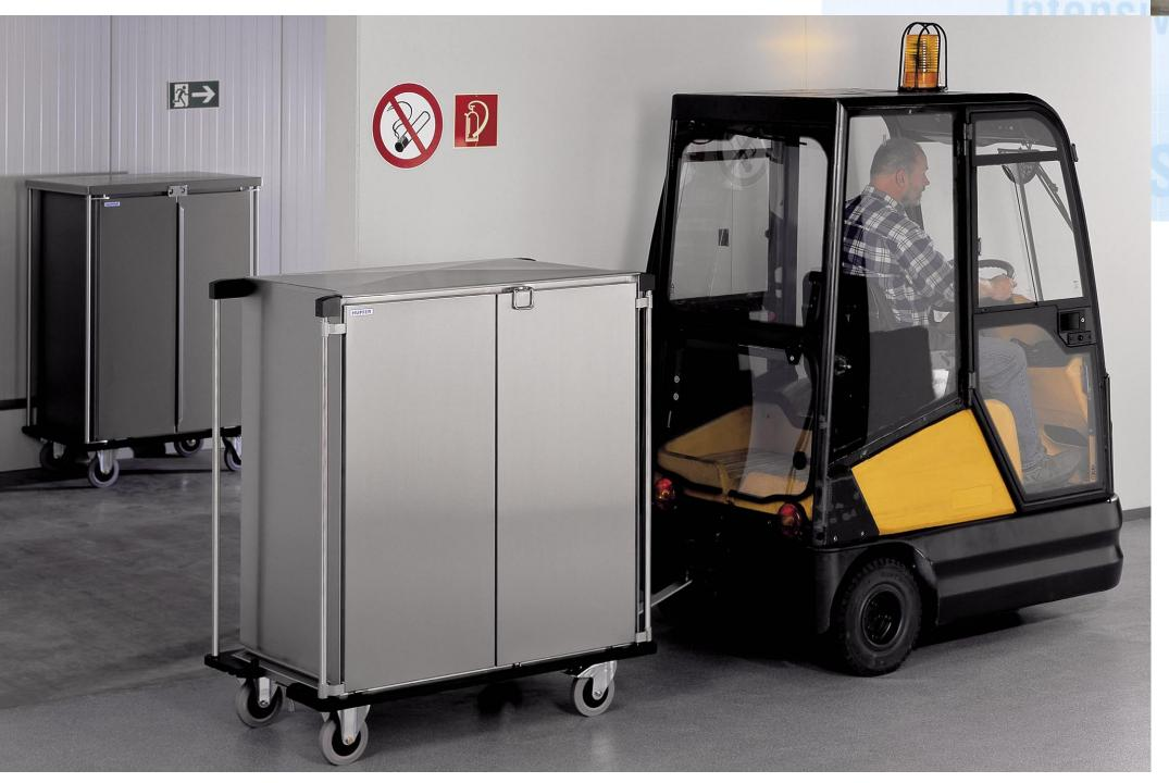
The HUPFER®ATW all-purpose transport trolley is suitable for in-line conveyance and can be adapted for use in automatic trolley transport systems.
