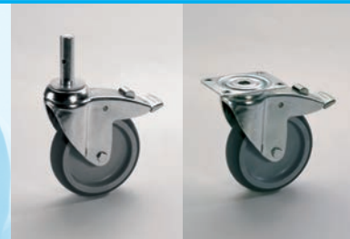
Rustproof castor in a galvanised-chromated housing with a plastic wheel and slide bearing as standard. Can be supplied with journal or plate attachment depending on the model.
