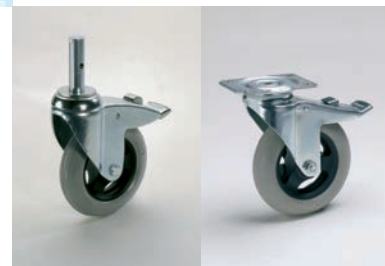
Rustproof castor with plastic wheel and smooth-running tread, ball bearing-mounted in galvanised-chromated housing. This type of castor ensures minimum travel noise and is especially suitable for running over uneven floors.
