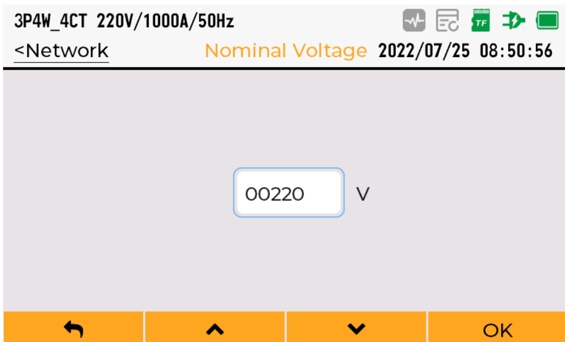
Figure 5-7 Nominal voltage configuration
