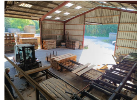
The sawmill first produced high-quality timber and uses the resulting off-cuts for the production of flooring at variable lengths, widths and grades. Customer buy a mix.
