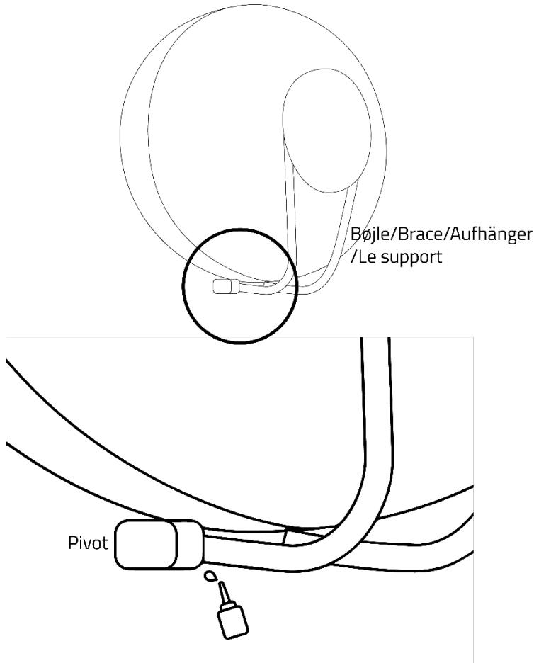
Lubricate occasionally pivot with one drop of acid free oil on each side for smooth operation.
