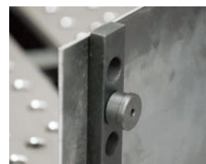
Magnet keeps sheet metal in vertical position
