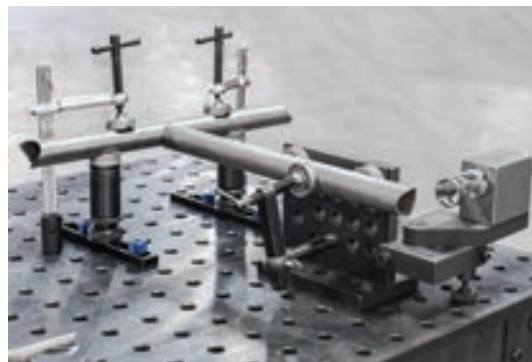
Arrange the Clamp and V-Blocks on the Modular Fixturing Block as needed for proper part positioning in each notching application.
