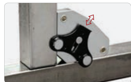
The face plate can be slid out of the boundary edges as edge guide.
