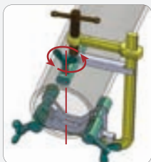
Turn three adjustment screws to preset.
