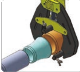
Pipe to Reducer
