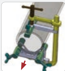
Loosen the main clamp arm.
