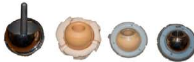
Figure 3.5: Different material combinations for the sliding pair, from left to right: 1. metall-metall, 2. ceramics-ceramics, 3. ceramics-polyethylene, 4. metall-polyethylene [Hop16]
