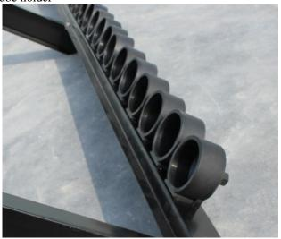
(4)Insert the bottom of water tank into the hole of frame, then, use the steel to stick it
