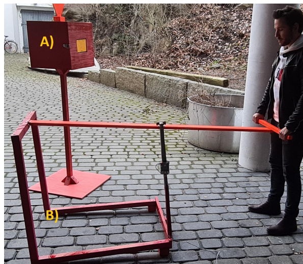
Figure 11 - Digital outdoor gym prototype with interactive hub (A) and digital training machine (B).
