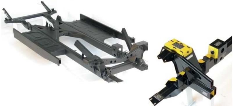
Our new **Austin Healey 100S** chassis and aluminium inner body panels made to exact specs.
